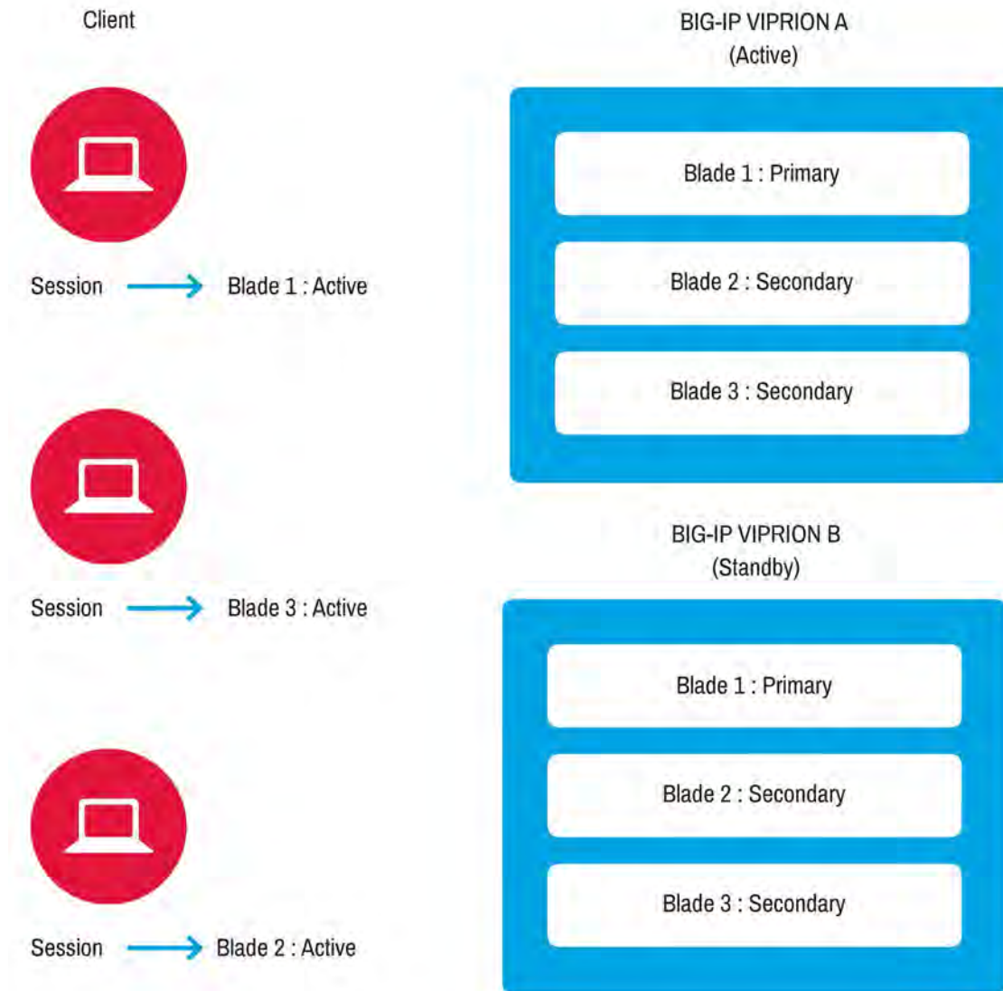
Figure 6.4: Active-standby VIPRION device group with all blades online
